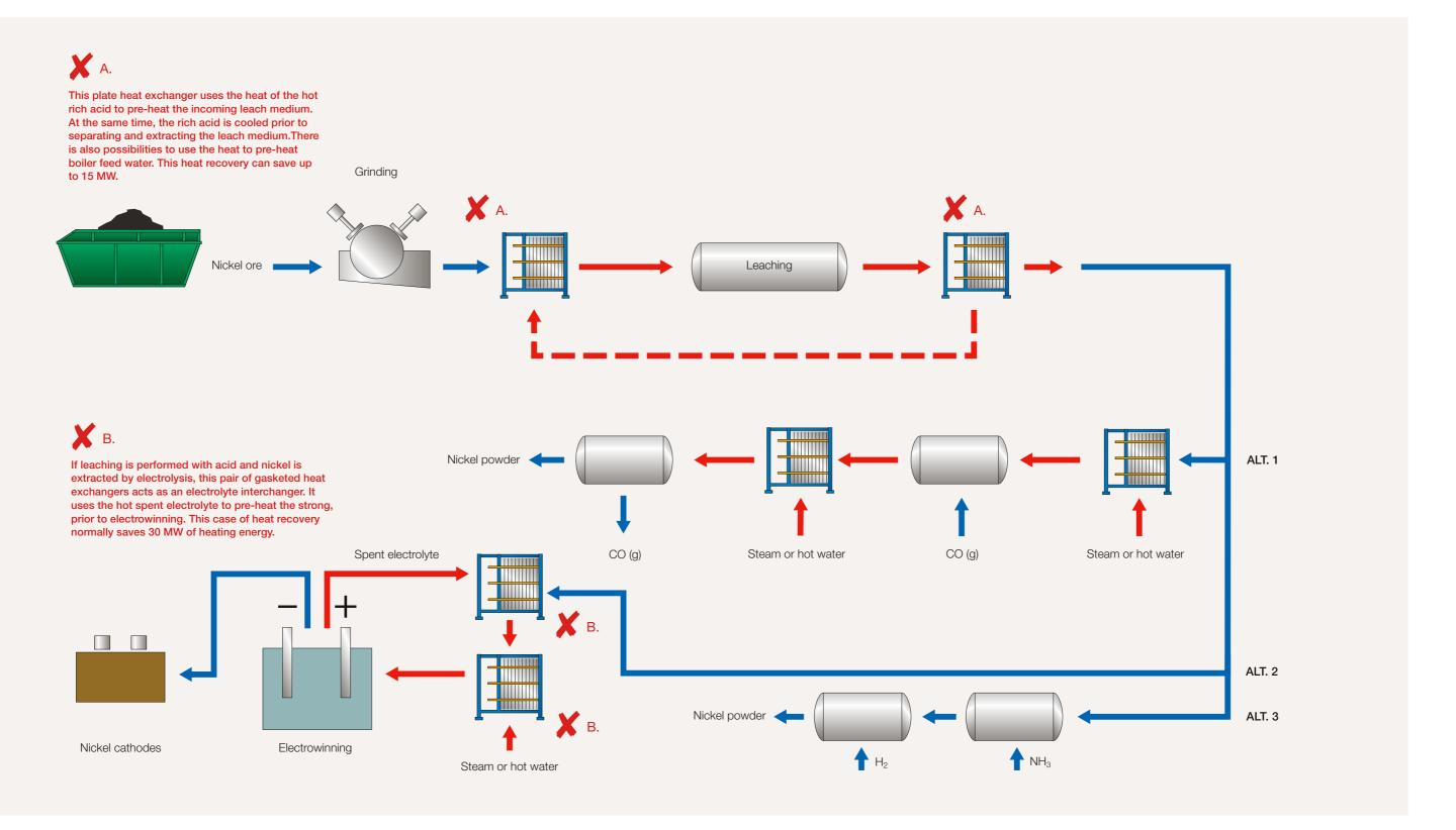
In nickel production, acid leaching, electrowinning and other energy-intensive extraction processes can be tapped for vast amounts of heat. Heat that can be fed right back into the flow, with an unparalleled yield.
