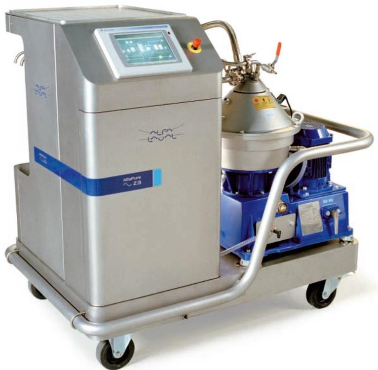
The choice of separator is governed mainly by the volume of the tank and the type of machining being performed. Alfa Laval's product range includes some ten separators, from the compact and mobile Alfie model to stationary models with a larger capacity.
