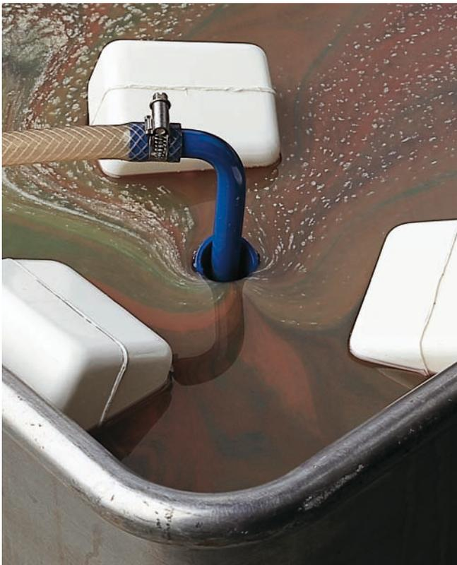
The contaminated coolant is skimmed from the surface.
