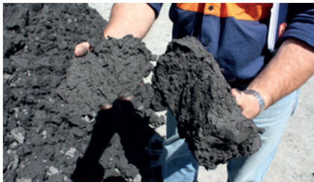
The Alfa Laval decanter produces spadeable cake with 67% dry solids by mass, which is put back into the open cut for mine rehabilitation.
