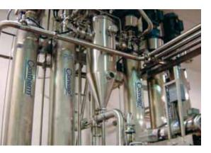
The lecithin is then separated from the vapours in a large cyclone, under vacuum, before being sent to Contherm heat exchanger(s) for cooling with water.
